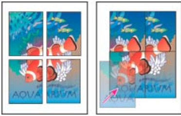
Oversized pages divided into printable tiles (left) and the overlapping sections in final assembly (right)
