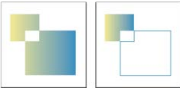
Gradient applied to a compound shape (left) compared to gradient applied to one part of the compound shape (right)
