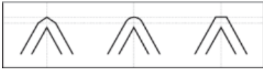
Trap join examples, left to right: miter join, round join, bevel join
